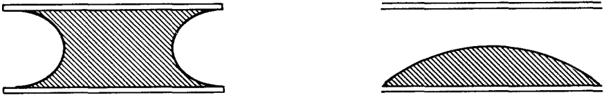
Fig. 4. Discontinuous behavior of a liquid drop bounded by two wetted plates. The instability is associated with the up and down directions contributing negatively to the surface energy.
